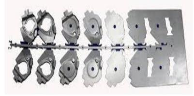
action required for a completed part. Even using multiple presses, secondary machining services were often required to truly complete a part. For that reason, progressive die stamping is the ideal solution for **metal parts with complex geometry** to meet:
