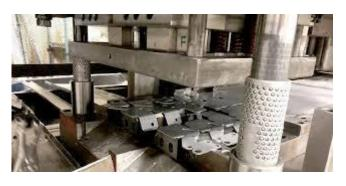
and avoiding burrs, which can drive up the cost of your part and extend lead time. The step is where you determine hole diameter, geometry/taper, the spacing between edge-to-hole and insert the first piercing.
