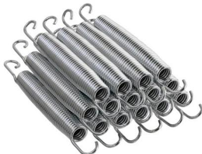
**(3" SPRING)** The 3" Rebounder Spring is approximately 3" long from the inside of the hook on one end to the inside of the hook on the other end. It has about 15 coils and an outside diameter of about 7/8". The total overall length of the spring from the outside of each hook is approximately 3 1/2".
